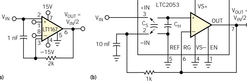
Practical implementations of the circuit in Figure 1 use the LT1167 (a) and the LTC2053 (b).
