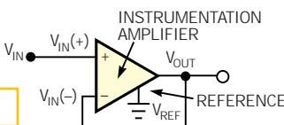
An instrumentation amplifier makes a simple divide-by-2 circuit.
